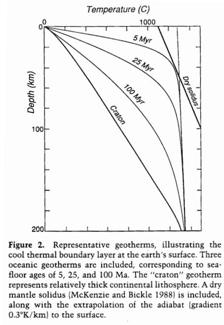
**Figure 2.** Representative geotherms, illustrating the cool thermal boundary layer at the earth's surface. Three oceanic geotherms are included, corresponding to sea-floor ages of 5, 25, and 100 Ma. The "craton" geotherm represents relatively thick continental lithosphere. A dry mantle solidus (McKenzie and Bickle 1988) is included, along with the extrapolation of the adiabat (gradient  $0.3^\circ\text{K/km}$ ) to the surface.
