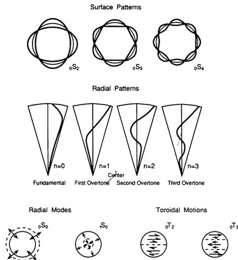
**FIGURE 4.24** (Top) Surface and radial patterns of motions of spheroidal modes. (Bottom) Purely radial modes involve no nodal patterns on the surface, but overtones have nodal surfaces at depth. Toroidal modes involve purely horizontal twisting of the Earth. Toroidal overtones ( ${}_{1}T_{2}$ ) have nodal surfaces at constant radii across which the sense of twisting reverses. (After Bolt, 1982.)
