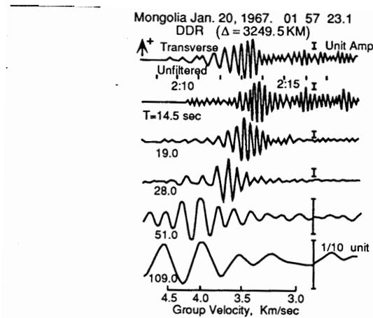
**FIGURE 4.26.2** Wave packets in narrow frequency bands obtained by filtering a Love-wave recording. The unfiltered record is shown at the top. Narrowband records with central periods shown on the left are plotted below the original seismogram, with varying amplitude scale. Note that each narrowband-filtered trace has the appearance of a wave packet. (From Kanamori and Abe, 1968.)
