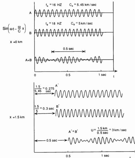
**FIGURE 4.12** Example of the interference of two waves of the form (4.36) at two positions  $x=0$  and  $x=1.5$ . The envelope of the interference pattern moves with group velocity  $U=3$  km/s. (Courtesy of H. Kanamori.)
