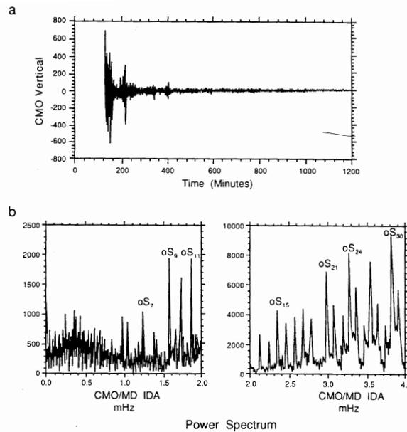
**FIGURE 4.23** (a) A 20-h-long record of an IDA gravimeter, CMO (see Chapter 5), at College, Alaska recording the 1985 Mexico earthquake. Long-period Earth tides have been removed. The bursts of energy correspond to Rayleigh-wave great-circle arrivals. (b) The power spectrum for CMO showing spikes at discrete frequencies corresponding to eigenfrequencies of the Earth. (Modified from Gubbins, 1990.)
