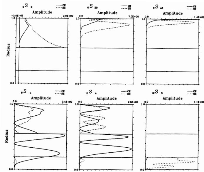
**FIGURE 4.25** Compressional (solid line) and shear (dashed line) energy density for fundamental spheroidal modes (top row) and some spheroidal overtones that are sensitive to core structure. (Modified from Davis, 1989.)
