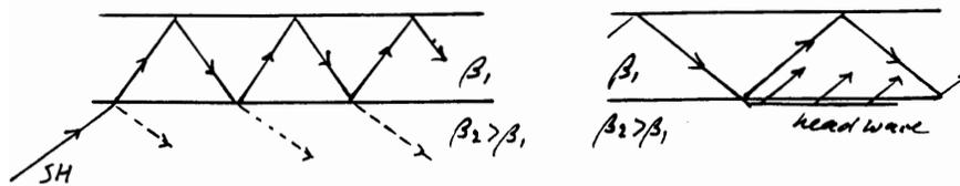
Figure 4.22: Trapped waves in the crust.
