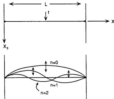
**FIGURE 4.22** Geometry of a string under tension with fixed end points separated by distance  $L$ . Motions of the string excited by any source ( $\mathbf{f}$ ) comprise a weighted sum of the eigenfunctions, which are solutions that satisfy the boundary conditions with discrete eigenfrequencies. The first three eigenfunctions are shown below.
