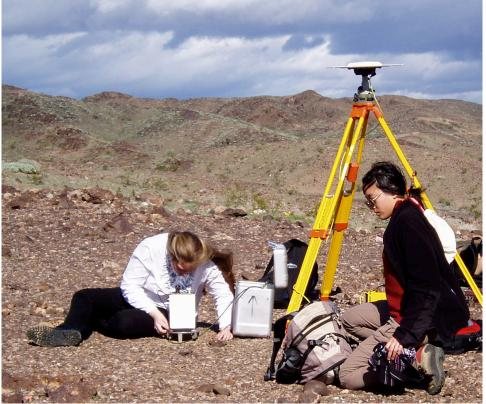
Figure 1: Using the gravimeter in the field
